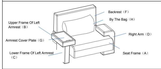
This chair has multiple parts and may require up to some 30 minutes to assemble. To give you an overview of the chair parts, the above picture is to help you put the various parts into perspective. Please read through the instructions below to familiarise yourself with the parts and steps before assembly.
