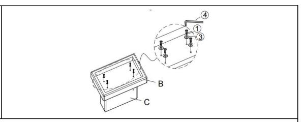
Attached upper frame of left armrest (B) to lower frame of left armrest(C) by using Bolt (1), Flat Washer (3) and Allen Wrench (4), as pictured above.
