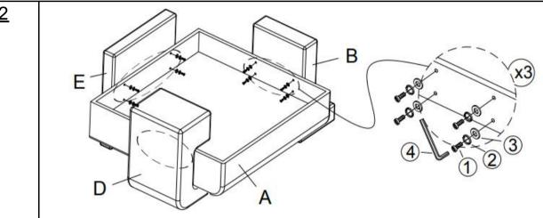
Attached upper frame of left armrest (B), right armrest (D), and rear leg(E) to seat frame (A) by using Bolt (1), Spring Washer (2), Flat Washer (3) and Allen Wrench (4), as pictured above.
